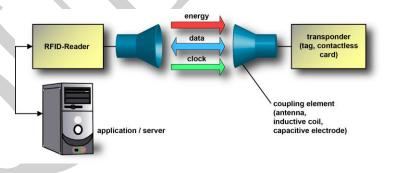
Figure: 4 Radio Frequency Identification
