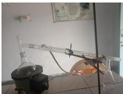
Scheme I: Distillation set-up used for distillation of Rum sample.
